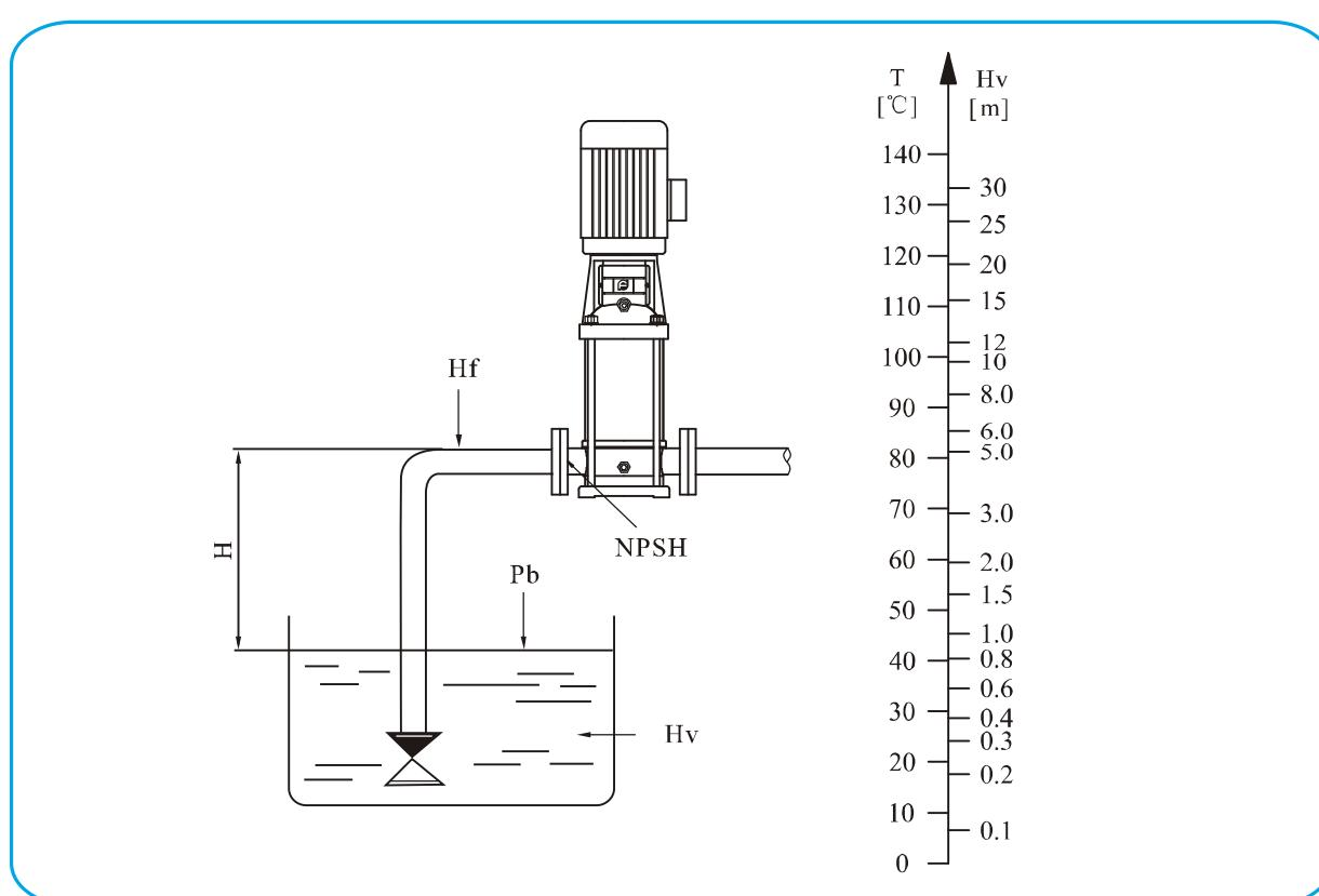
Check and ensure that the pump is not at cavitations state.
